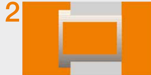
2 Assembly iglidur® plain bearing with sliding fit
