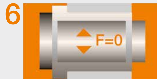
6 Result: low clearance bearing despite "inaccurate" hole/pin
