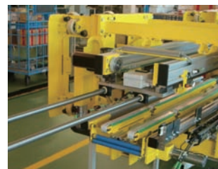
存储滑动单元自动存储/检索系统 Storage-slide unit for an automatic storage/retrieval system
