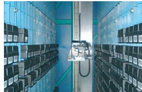
DryLin® W 用于高架仓储设备 - 提升轴 DryLin® W in high-rack facilities – Application: Lift axis
