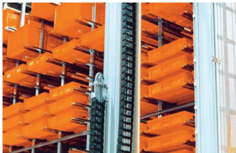
中等尺寸的拖链用于高架仓储设备 e.chains® in medium size in storage and retrieval machines
