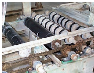
耐脏污: igubal® 基座轴承用于石材加工 Resistant to dirt: igubal® pillow block bearings in stone processing
