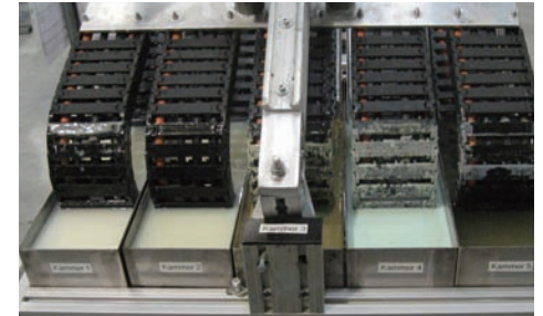
介质测试: 化学介质中的耐久度测试 Media test: Test of durability of chemical interferences in motion
