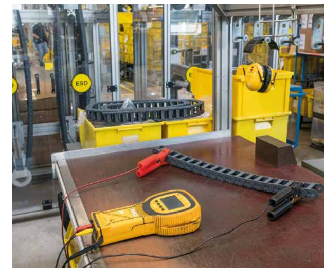
100% of the produced igus® ESD e-chains® are checked for their continuous conductivity from one end to the other
